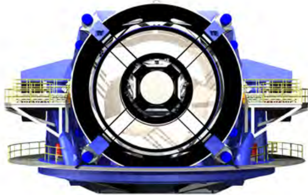
FIGURE 7.8 LSST has a three-mirror design with the primary and tertiary mirror combined and cast from a single blank. Preliminary grinding is already underway and the secondary mirror has also been cast. An important figure of merit for a survey telescope is the etendue, which is the product of the field of view and the area. This is 320 \text{ m}^2 \text{ degree}^2 for LSST. The 3 GPa camera will read out in less than 2 seconds every 15 seconds, and more than 100 petabytes of data will be accumulated over the 10-year project lifetime. The limiting magnitude in a single visit is r = 24.5 . The camera pixel scale is roughly 0.2 arcsecond, and the median seeing at the site is roughly 0.67 arcsecond. Credit: LSST Corporation.
