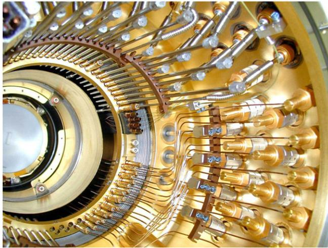
**Figure 10.** Upper end of cryogenic Probe showing gold-coated leads and surfaces to reduce radiation and in lower left the first radiation window connected to the vapor-cooled shield.
